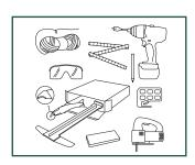
The following standard tools are needed: hammer, saw with blades for plastic (a jigsaw, hand circular saw, hand saw, or cross-cut saw), mouth mask (during sawing), measurer, safety glasses, thin rope, gloves and a pencil. Besides that, you also need the following accessoiries: Pergo INSTALLATION SET (a pull-bar, spacers and a tapping block suitable for the Uniclic® click system), Pergo Rigid underlay system and suitable maintenance products.
