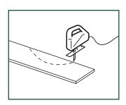
For any other cuts, you need to saw the planks. Depending on the type of saw, position your plank with the decor side face-up or face-down. Before making the actual cut, use a leftover piece to determine how the cleanest cut can be obtained (decor side face-up or face-down).
