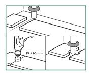
In rows where there is a pipe, make sure the pipe falls exactly in line with the short side of two planks. Take a drill bit with the same diameter as the pipe plus 16mm (0,63inch). Click the planks together on the short side and drill a hole centered on the joint between the two planks. Now you can install the planks.
