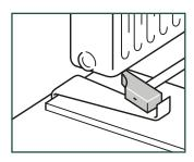
In places where it is difficult to install the planks with the tapping block (e.g.underneath radiators), you can tap them together with the pulling iron and a hammer.
