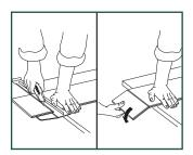
To shorten the length of the plank with a straight cut, you can cut the PERGO rigid vinyl floors with the decor side face up, using a special concave vinyl cutting knife. In order to cut the vinyl plank, draw a straight line along which you will be cutting, and use the knife to make a firm cut in the surface. You never need to completely cut through the vinyl. Then break off the plank using both hands.
