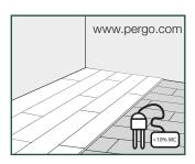
In case of installation on a wooden subfloor, please remove any existing floor covering first. No signs of mold and/or insect infestations should be present. If there is moist in the woodbased subfloor or there is no proper moisture barrier below the woodbased subfloor it has to be removed first. Reason is that the wood wil rot after time because the moist is blocked by the new flooring and its underlay.
