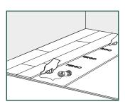
It is recommended to make additional checks of the straightness, in order to confirm the straightness during the installation. Remember to use the distance spacers for the expansion gap of 8mm (0,315 inch) along the perimeter.
