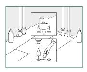
In rows where there is a double pipe, proceed as follows: 1. Measure where the pipe will come through the plank. Don't forget to allow room for the expansion joint. Measure the diameter of the pipe plus 16 mm for the expansion. 2. Drill through the panel where the pipe will come through 3. Extend the hole to the edge of the panel 4. Lay the panel around the pipe
