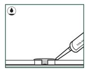
Push the Incizo profile in the base profile and the wet Sealant. Add Sealant where the Incizo touches the floor for a perfect waterseal.
