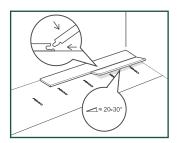
In order to make the start of the installation easier, assemble the first 3 rows away from the wall, so you can sit on the planks during the assembly. Then slide the first 3 rows at the wanted position close to the wall with distance spacers in place.
