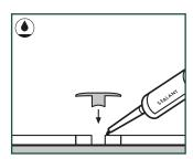
Fix the Incizo base profile to the subfloor with Pergo Multiglue. Apply the flexible Sealant on the PE foam that is in the expansion joint.
