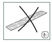
Check all panels before and during installation in optimal daylight conditions under the angle of light reflection. Defective panels must never be used. An installed plank is considered as accepted and cannot be claimed.
