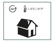
Pergo rigid vinyl has been designed for indoor heated (>  $5^{\circ}$ C) (41°F) installations, preferably at normal room temperature (=  $18 - 30^{\circ}$ C).
