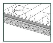
Floor heating systems (water / electricity) which are built-in the screed can be used with Pergo rigid vinyl floors if a constant room & floor temperature of minimum 18°C (64°F) can be guaranteed during acclimatization, installation and 48h after installation.
