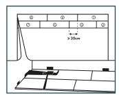
In places where it is too difficult to install the Unilic® planks with the tapping block (e.g. against the wall), you can pull them together using the pull-bar and a hammer.
