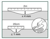
Cement joints between tiles or other gaps of more than 2mm (0,08inch) in depth and 5mm (0,2inch) in width should be levelled.
