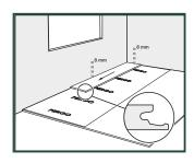
Start with the first plank that will be installed in the corner. Remove the click profile on both the long and the short side of the plank by sawing. For other planks of the first row (not in the corner), remove the click profile on the long side that will be directly next to the wall. Any side of a plank that is directly next to a wall, must have its click profile removed, in order to ensure the required expansion gap.
