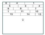
$\label{lem:continue} Continue the installation like this - row by row - towards the end of the room. \\ The easiest way to work is to sit on the already installed planks.$
