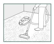
Make sure that the subfloor is dry, flat, stable, clean and free from grease and chemical substances. If needed, scrape off and clean up old adhesives. Prior to installation, carefully remove all debris (including nails), sweep and vacuum. Repair major surface imperfections and large cracks. It is recommended to remove old skirtings and to install new ones after the installation of the floor.
