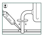
For a perfect finish around pipes, use Pergo radiators caps and the elastic waterproof transparent Pergo Sealant, taking into account the expansion of 8mm. Place the foamstrip in the expansionjoints. Apply Sealant on the foamstrip. Then place the pipe covers in a floating installation.
