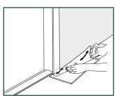
Do not fill or cover the expansion joints with silicone or other kit. If you would like to finish your floor fully waterproof, read the instructions below "3. FINISHING IN ROOMS LIKE BATHROOMS, KITCHENS, LAUNDRY ROOMS
